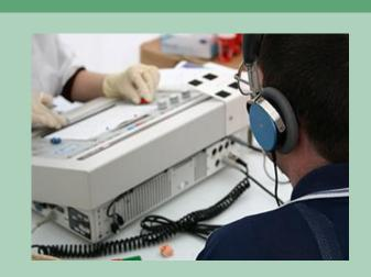
Among other specialized equipment an Audiologist will use an audiometer, which is a machine used for testing hearing loss.
